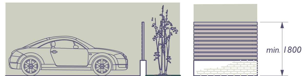
C3. Boundaries between dwellings and existing rear access road - Timber fence on low wall
